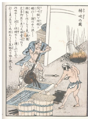
Casting cooper into bars [ copper freezing ] (Kodō Zuroku. Illustrated Book on the Smelting of Copper, 1801)
